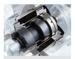
Uncompromising sealing technology for very demanding applications. Hermetically sealed magnetic couplings guarantee leakage-free and maintenance-free pumping and mixing. The media remains within closed system circulation loops.
