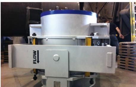
An Australian refinery has been fitted with a **cold wall gimbal expansion joint** ( $d = 1,067 \text{ mm (42")}$ ) and a **tied universal single expansion joint** ( $d = 889 \text{ mm (35")}$ ). Operating conditions:  $p = \dots 4.14 \text{ bar (60 PSI)}$ ;  $t = 750 \text{ }^\circ\text{C (1,382 }^\circ\text{F)}$ . Medium: flue gas.
