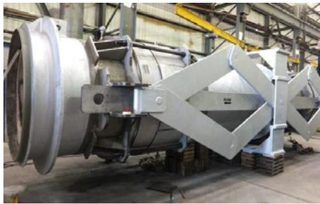
EagleBurgmann provided a large sized **universal spent catalyst standpipe expansion joint** for a refinery in Texas, USA. Operating conditions:  $p = \dots 3.79 \text{ barg (55 PSIG)}$ ;  $t = 732 \text{ }^\circ\text{C (1,350 }^\circ\text{F)}$ ;  $d = 1,500 \text{ mm (59")}$ . Media: flue gas and catalyst fines.
