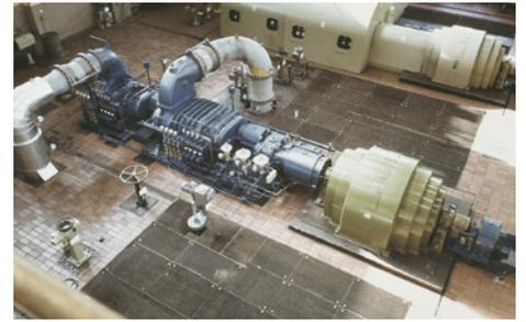
The two-stage screw compressor (Aerzen VR0825) used to compress coking oven gas in a coking plant is one of the biggest ever built. It is sealed with an EagleBurgmann type **HSH2/215**.
