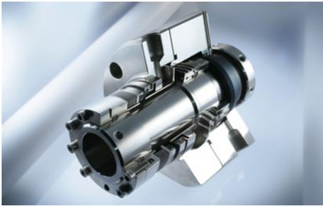
An EagleBurgmann **MFLWTS1/83** seals the shaft of a Leistritz screw pump in the de-asphalting unit of the ENI refinery in Sannazzaro de' Burgondi, Italy. Pump and metal bellows seals were started up in 2006. Operating conditions:  $p = 1.87 \text{ bar (27 PSI)}$ ;  $t = 274 \text{ }^\circ\text{C (525 }^\circ\text{F)}$ ;  $n = 1,700 \text{ min}^{-1}$ ;  $d1 = 75 \text{ mm (2.95")}$ . Medium: asphaltene.
