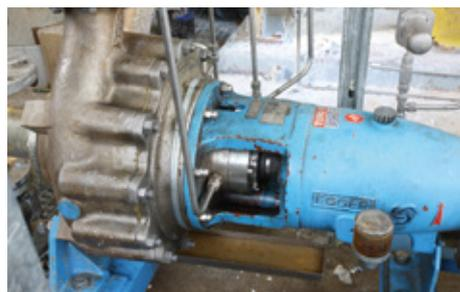
Centrifugal pumps at Polymer-Latex GmbH in Marl, Germany, are successfully sealed with **Cartex-DN** type seals. The process medium – a latex dispersion – represents a challenge for the seal. The **FLC200** flow rate control unit supplies and flushes the seal.
