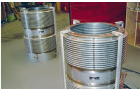
The El Dorado Chemical Co. in Arkansas, USA, uses **metal expansion joints** in the plant for manufacturing nitric acid. Operating conditions:  $p = 10\text{ bar}$  ( $145\text{ PSI}$ );  $t = 649\text{ °C}$  ( $1,200\text{ °F}$ ).
