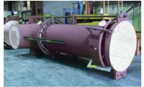
Several **metal expansion joints** are employed in the ethylene cracker at Nova Chemicals in Sarnia Ontario, Canada. Operating conditions:  $p = 3.45\text{ bar}$  ( $50\text{ PSI}$ );  $t = 420\text{ °C}$  ( $788\text{ °F}$ ).
