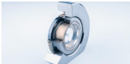
Gas-lubricated **MFLC-GS** metal bellows seals as single or double seals for the shafts of process pumps in air separation plants. Typical process media are liquefied gases such as nitrogen. The low temperatures require special materials for the secondary seals, such as the proven **Statotherm** graphite seals. Operating conditions:  $p = \dots 25 \text{ bar}$  (363 PSI);  $t = \dots -199 \text{ °C}$  (-326 °F);  $n = 6,000 \dots 8,000 \text{ min}^{-1}$ .
