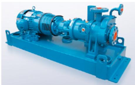
A Roth pump, sealed with a **MAK66** magnetic coupling, in use at a manufacturer of soap and cleaning agents in the US. Operating conditions:  $p$  = 22 bar (319 PSI);  $t$  = 50 °C (122 °F);  $n$  = 3,500 min<sup>-1</sup>.
