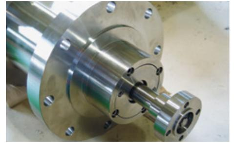
Bayer in Leverkusen, Germany, uses several screw spindle pumps to manufacture preproducts for polyurethane production that are sealed with **MAK66S3** type magnetic couplings. The process media are various polyethers with viscosities up to 3,500 mPas. Operating conditions:  $p = 6\text{ bar}$  ( $87\text{ PSI}$ );  $t = 20 \dots 80\text{ °C}$  ( $68 \dots 176\text{ °F}$ );  $n = 350 \dots 1,500\text{ min}^{-1}$ .
