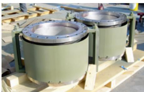
Dupont de Nemours and Company in Pass Christian, USA, uses several **expansion joints** in steam / colored pigment production. Operating conditions:  $p$  = +0.48 ... -0.48 bar (+70 ... -70 PSI);  $t$  = 354 °C (669 °F).
