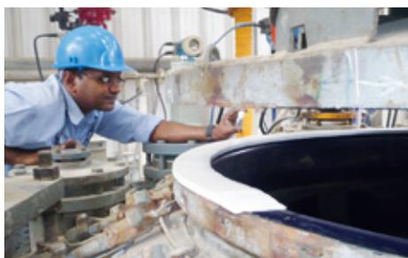
Tytan Organics Chemical Co. in the United Arab Emirates uses glass-lined reactor vessels to manufacture concrete plasticizers. The flanges and covers are sealed with **Burachem multi-gaskets** made from pure PTFE. Medium: Naphthalene sulphonate formaldehyde. Operating conditions:  $p$  = 6 bar (87 PSI);  $t$  = 220 °C (428 °F).
