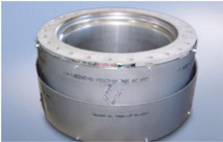
The Columbian Chemicals production facilities in Centerville, USA have a number of **expansion joints** installed in the exhaust gas system. Operating conditions:  $p = 0.35 \text{ bar}$  (5 PSI);  $t = 760 \text{ }^\circ\text{C}$  (1,400  $^\circ\text{F}$ ).
