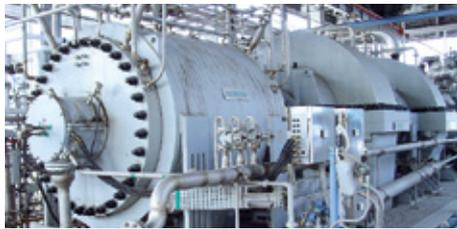
Sealing a coolant compressor at the Yeochun NCC Company in Korea with a **PDGS10** – a gas-lubricated multiple mechanical seal in tandem arrangement. The medium to be sealed is ethylene. Heat tracing at temperatures down to  $-100\text{ }^{\circ}\text{C}$  ( $-148\text{ }^{\circ}\text{F}$ ) is unnecessary due to the application of a special dynamic secondary sealing element.
