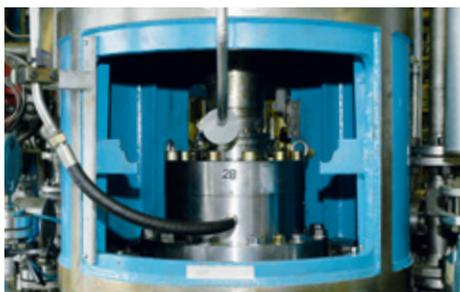
Wacker Chemie AG in Burghausen, Germany, seals a number of top-drive high pressure reactors for polymer dispersion manufacturing with **HSHLV-D** type high pressure seals with cooling flange. A shared buffer system supplies all the seals. Operating conditions:  $p_1$  = vacuum ... 100 bar (1,450 PSI);  $t$  = ... 100 °C (212 °F);  $n$  = 25 ... 100 min<sup>-1</sup>.
