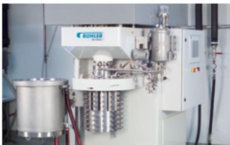
A Korean chemical company seals its Bühler bead mills for paint production with **MR1S1F-D24** type mechanical seals. The process medium – colored pigments with various solvents – is very abrasive.
