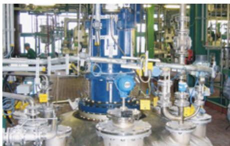
Sealing of polymerization reactors with an **HSMR5L-D** in the manufacture of synthetic rubber at Lanxess Deutschland GmbH. The process medium – monomers, water and polymers – has a tendency to bond. So flushing is used to protect the seal. An **SPA4025** buffer pressure system is used as the supply system.
